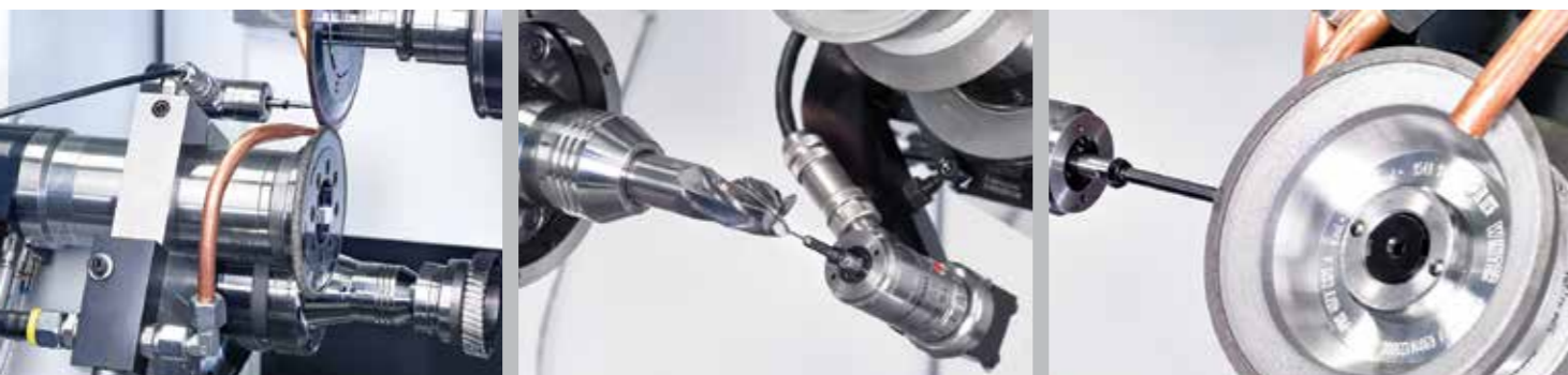
Dressing attachment that saddles the workpiece axis (A-axis)
