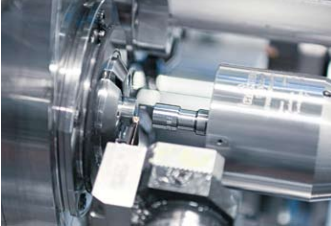
Workpiece parting off and takeover by the opposed spindle
