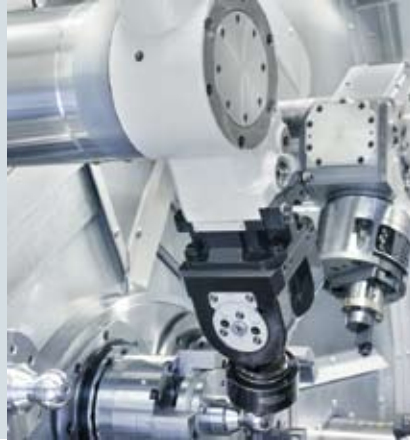
Spherical finishing tool installed on a 1-position machining unit
