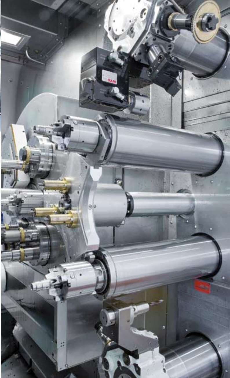
Two-side machining with three fully-fledged additional spindles and up to eight tools
