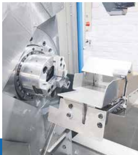
Parts discharge via chute
